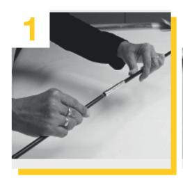
Please join the glass fibre rods for the upper and lower ring.
